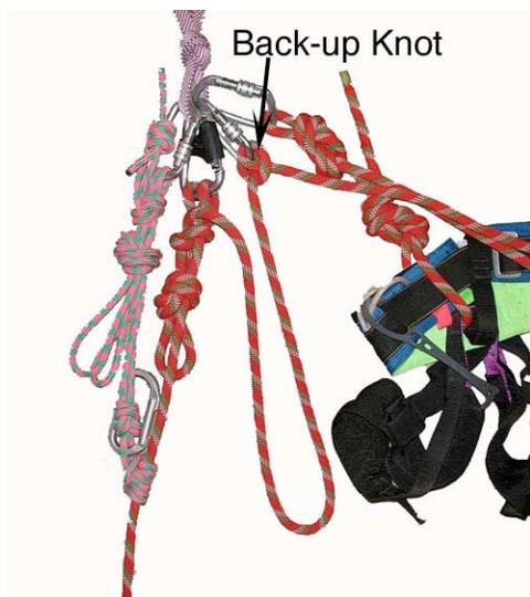
**Step Six:** Using another separate carabiner tie the main rope coming from the belay device directly onto the anchor leaving about 30 – 50cm of slack. This acts as a back-up while allowing enough free rope to be available to rig a pulley system or other rescue system. (Note this step can be performed before attaching the Prusik cord.)
