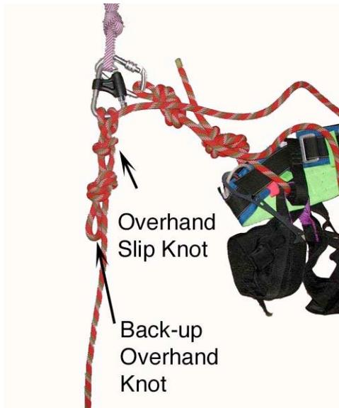
**Step Four:** Using the bight of rope that exits from in front of the slip knot, tie an overhand knot as a back-up. At this point you have effectively escaped the system and can proceed to make decisions regarding what action to take next.
